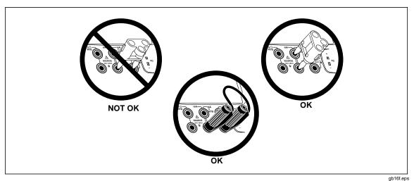
Figure 16. Proper and Improper Jumper Use
