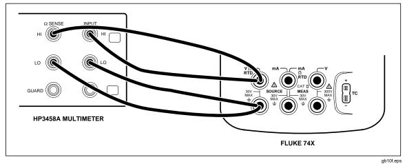
Figure 9. Resistance Source Verification Connections
