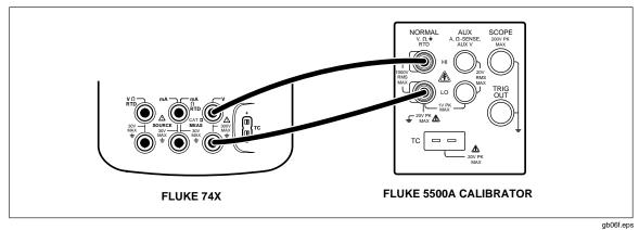
Figure 5. Frequency Measurement Verification Connections
