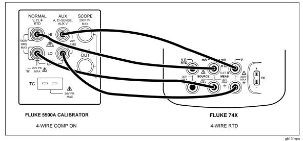
Figure 12. Four-Wire RTD Measure Verification Connections
