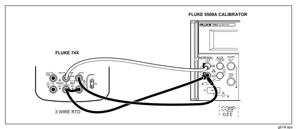
Figure 13. Three-Wire RTD Measure Verification Connections
