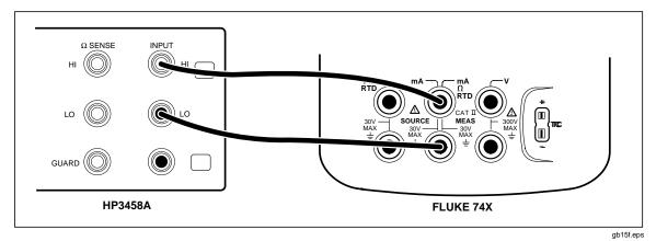
Figure 14. Loop Power Verification Connections
