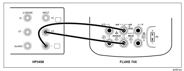
Figure 7. DC Current Source Verification Connections
