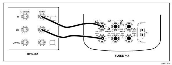
Figure 6. DC Volts Source Verification Connections
