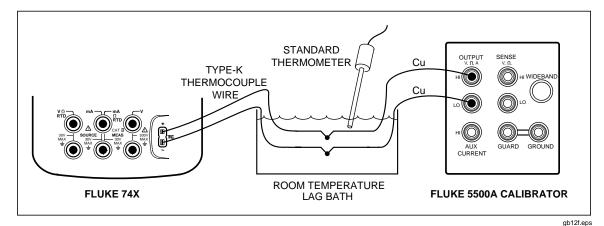
Figure 11. Temperature Measure (TC) Verification Connections
