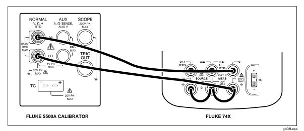
Figure 2. DC Volts and AC Volts Measurement Connections
