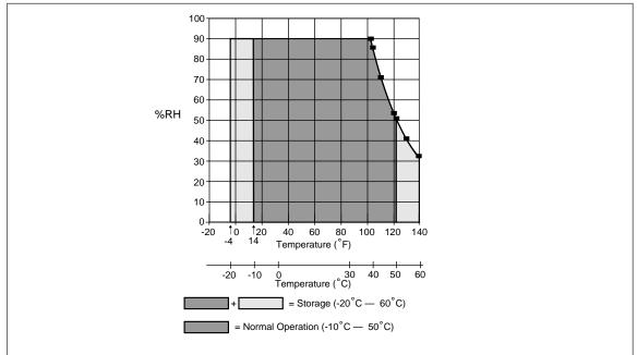
Figure 1. LCD Operating Environment Specification
