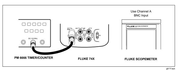
Figure 10. Frequency Source Verification Connections
