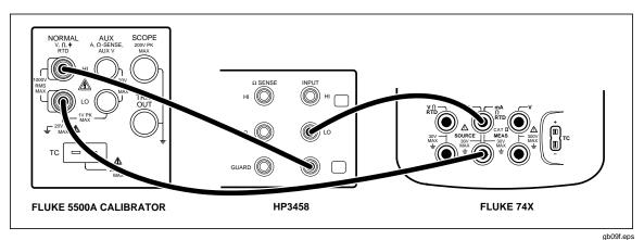
Figure 8. Simulate Transmitter Verification Connections
