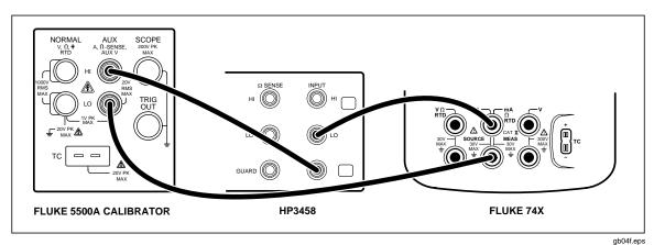
Figure 3. DC Current Measurement Verification Connections
